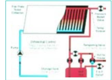
Open loop forced circulation systems transfer heat directly to water to be used. When water in the collector loop is hotter than the water in the storage tank, the pump is activated and water from the tank is circulated through the collector.
