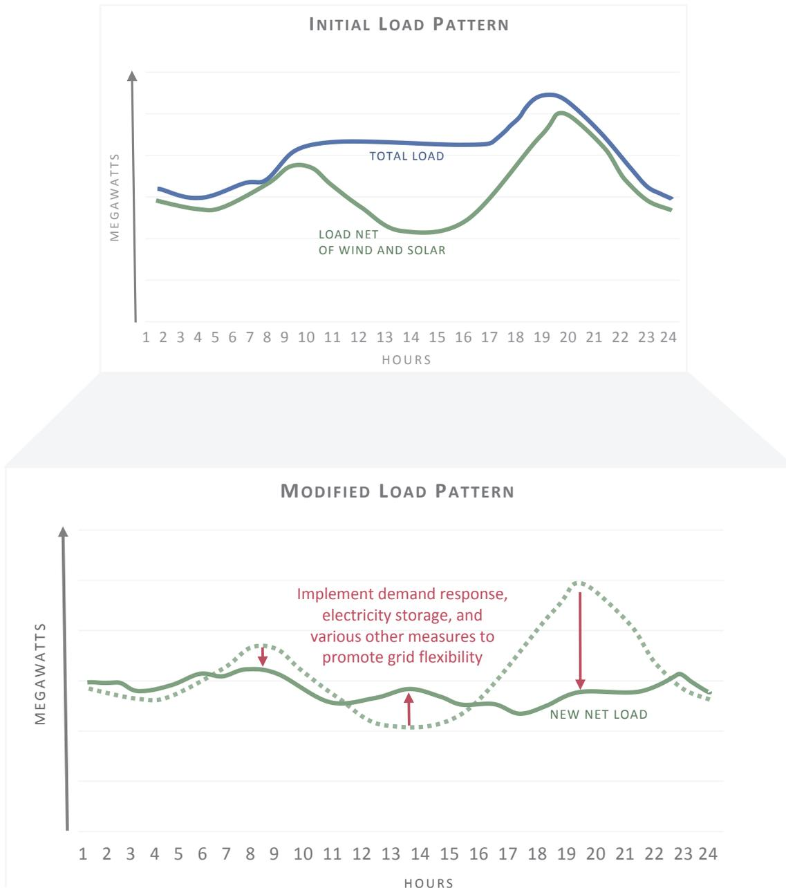
*Note: Flexibility measures can reduce the need to rapidly ramp dispatchable generation to meet load net of variable wind and solar generation. Flexibility measures include demand response, targeted energy efficiency, peak-oriented renewables, storage, better forecasting and planning especially for variable renewable energy, inter-regional power exchange, and replacement of inflexible generating units with flexible generating units. Source: Adapted from Lazar 2016, Figure 5.*
